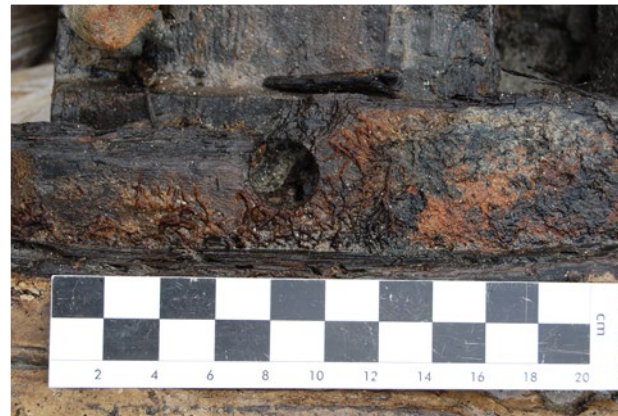
Detail of the pitch that coated the hull and remains of the moss used to seal the joints. SAB
