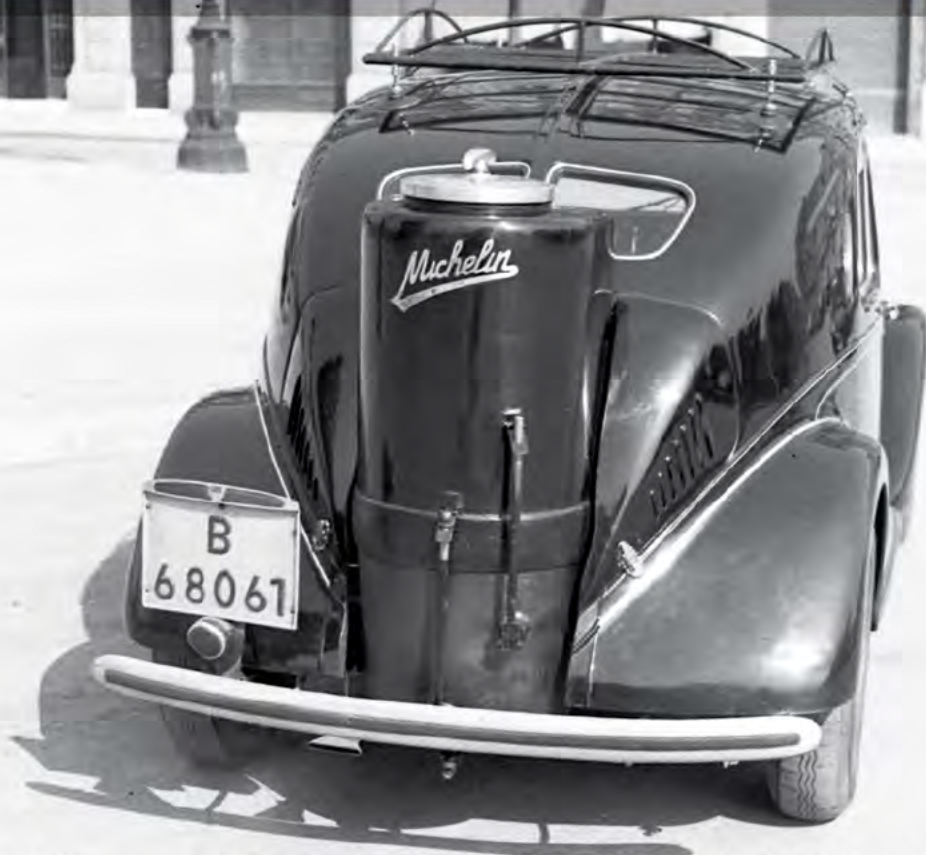
Car fitted with a gasogene made by Roig i Pérez. Photograph by Brangulí (photographers), 1940-45. ANC
